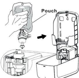
SECURE THE PUMP WITH CLAMPS AND MAKE SURE IT IS LOCKED IN THE SLOT. REPEAT STEP 9-11 FROM USER MANUAL.
