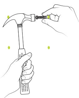
TAP ANCHORS INTO EACH DRILLED HOLE.
